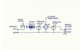
The Rx is 27 MHz from a toy, motor needed 9 volts, sound card needed 5 volts, hence voltage regulator.
