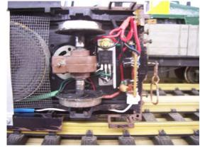
The sound card emits a constant CHUFF, 0.25 Watt 50mm speaker is mounted under footplate.
