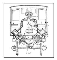
Some unique features of this 0-4-0 version Heisler include; the V2 cylinders under the boiler immediately in front of the firebox at footplate level, the cylindrical water tank on footplate, the wood burner fuel is stored at the back deck, covering the 9 volt battery.
